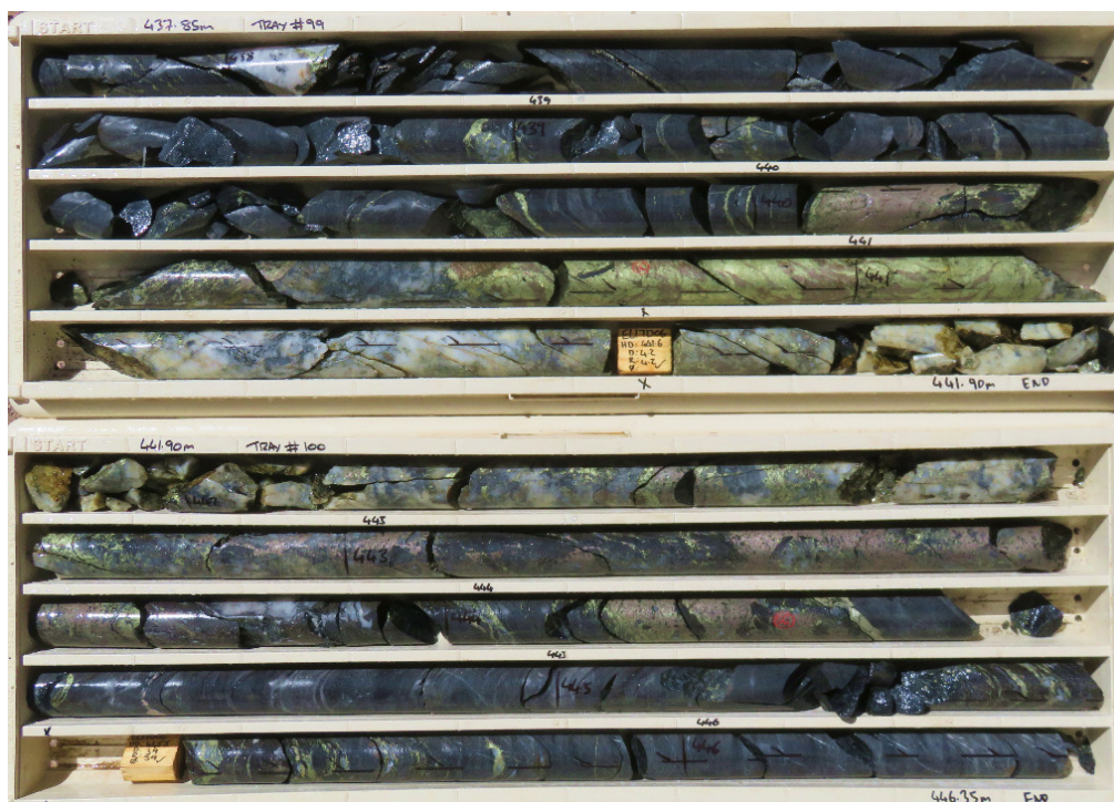
Figure 4: EL17D06: mineralisation between 437.85-446.35m. Sulphide is mostly chalcopyrite (yellow) with lesser pyrrhotite (bronze in colour)
