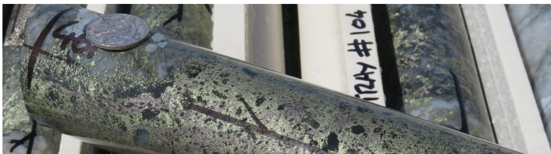
Image: Massive chalcopyrite and pyrrhotite from hole EL17D06 at 461m
