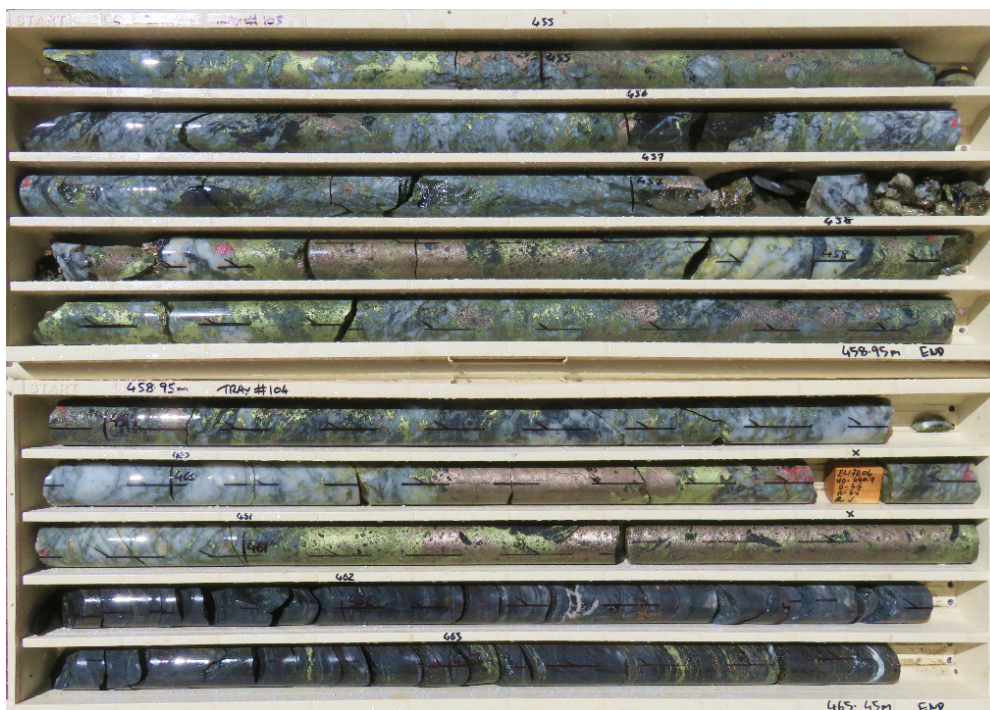
Figure 5: EL17D06: mineralisation between 454.5-463.45m. Sulphide is mostly chalcopyrite (yellow) with lesser pyrrhotite (bronze in colour)
