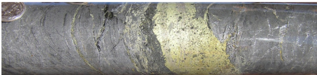
Figure 2: Chalcopyrite + pyrrhotite vein at 246.3m in DD16TUR016 from the Bellatrix EM conductor within the Skylark Shear Zone
