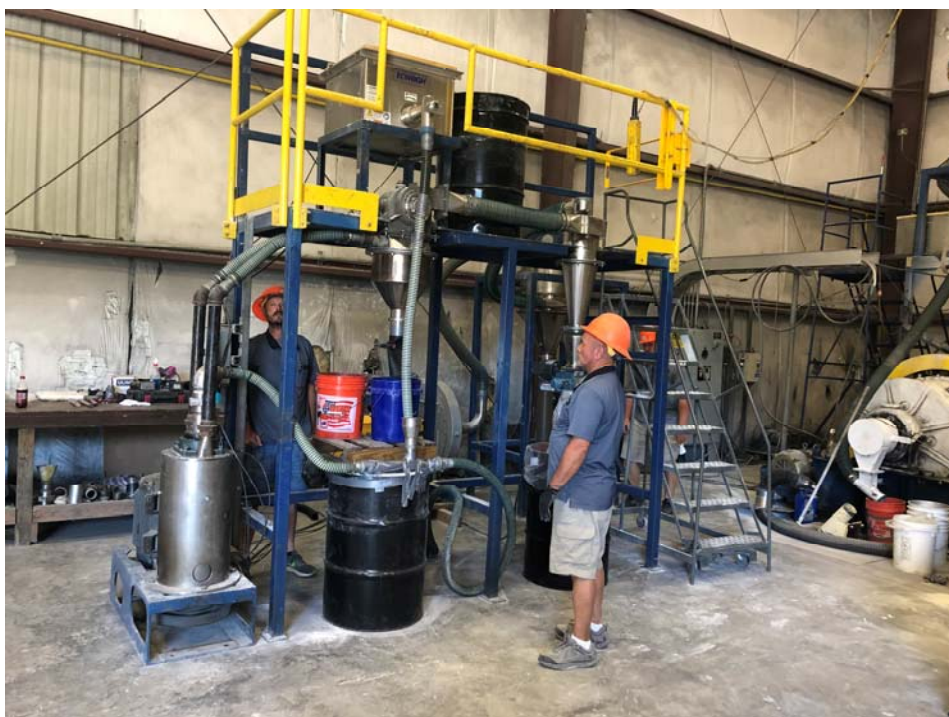
Figure 3: Dry processing trials performed on Carey's Well ore by USA leader in kaolin plant design
